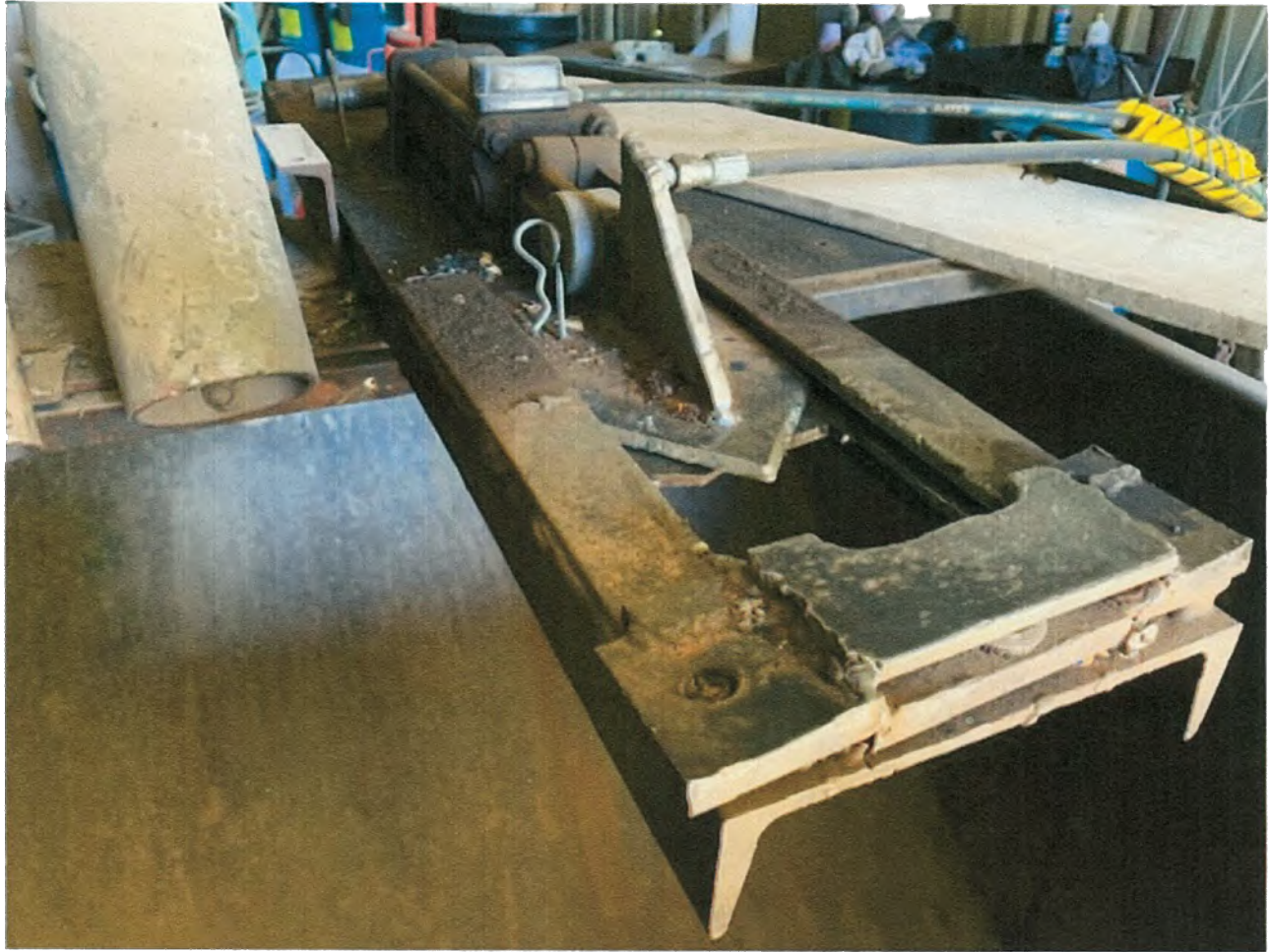
This picture shows the hydraulic metal shear that is used to cut or put a hole in the green propane. This machine will be getting updated soon.
