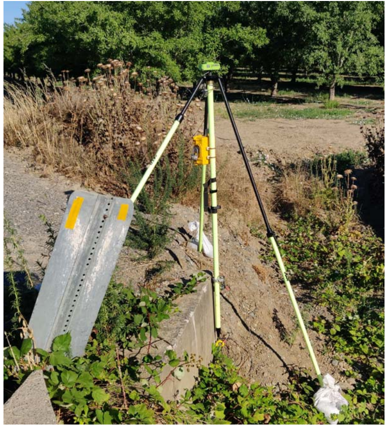
RTK base receiver at 5B35
