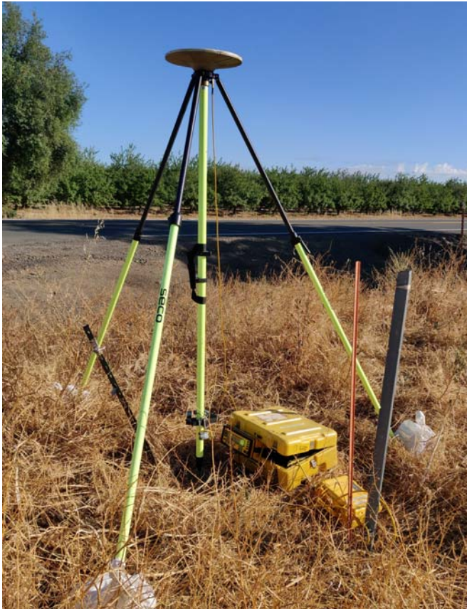
Static GPS receiver at H62U
