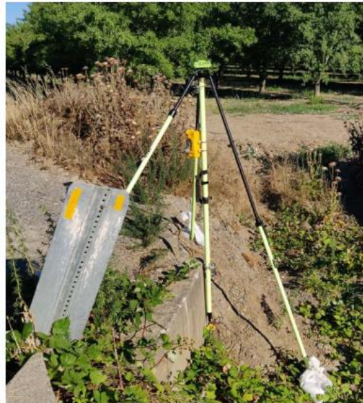
RTK base receiver at 5B35
