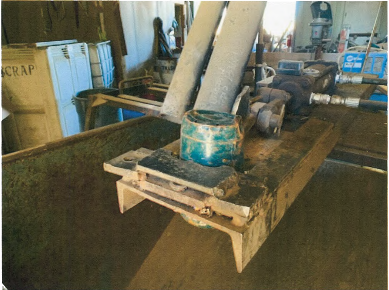
You can see the green propane tank in the shear ready to be cut in half or have a hole put into it.
